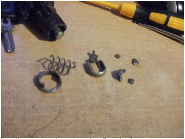
**Step8**: This is the parts of my lock once I removed it, you'll notice the broken bits which was causing my problems (castle). I simply needed to replace this part to repair mine.
