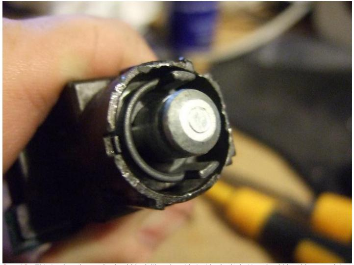
**Step10**: This is what the castle should look like when it's inside the lock. You should be able to work it out when fitted, as the castle has two locator holes which fit over the lock holes and there is a small notch which aligns with the missing section on the lock. I've tried to show it here
