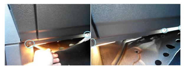
When you have removed the torx screws (I have circled their relevant positions above) and the flathead screws from the foam, you will need to remove the foam away from the covers. I found the best way to do this is by digging a finger just behind the light, there is a gap here. Once you have started moving the foam away it should come off easy if you have removed all 5 screws.
