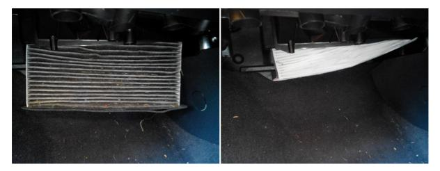
After the old filter has dropped down when the cover was removed (picture above) all you have to do is reinstall the new filter, it should slot in easy enough, just reinstall in the same procedure the old one came out (for reference it reinstalls in the orientation in the picture below)
