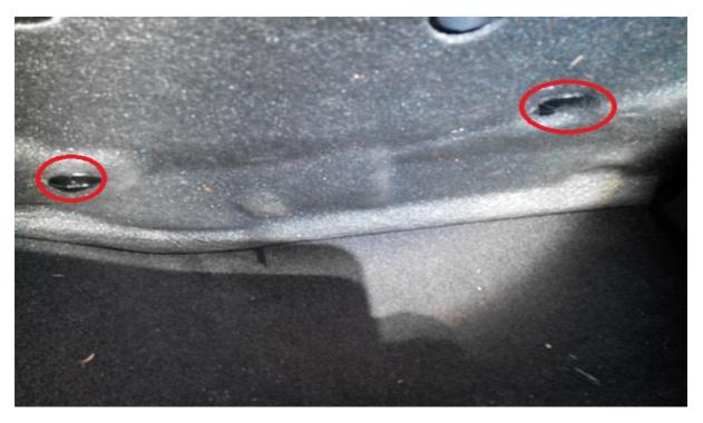
When you have removed the Torx screws, change your bit or changeover to the flat head screwdriver. You will need to look underneath the glove box; you will then see the following two plastic screws holding the foam in place. Remove these screws
