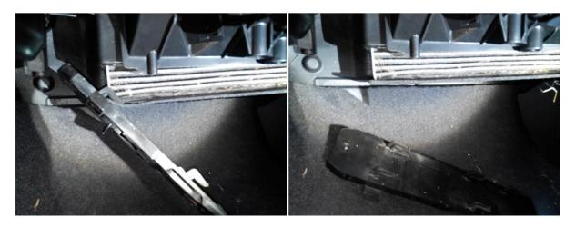
When you have slid the cover off, it will fall down to the floor and the older filter should pull out quite easy enough. You will then be able to see the quality of the filter you are removing on your car after the latch has been released
