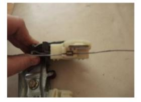
The small tab on the metal wire needs placing into the appropriate hole on the plastic window holders
