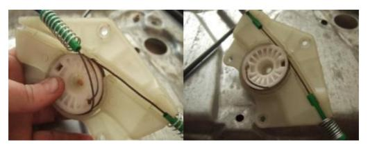
After you have wrapped the wire around the wheel, you will need to put it inside the housing with the inside edge with the teeth facing outwards. You will then need to compress the springs on the plastic tabs against the housing so that everything fits. This step will be <u>HARD</u> to some degree if not using a pretensioned kit
