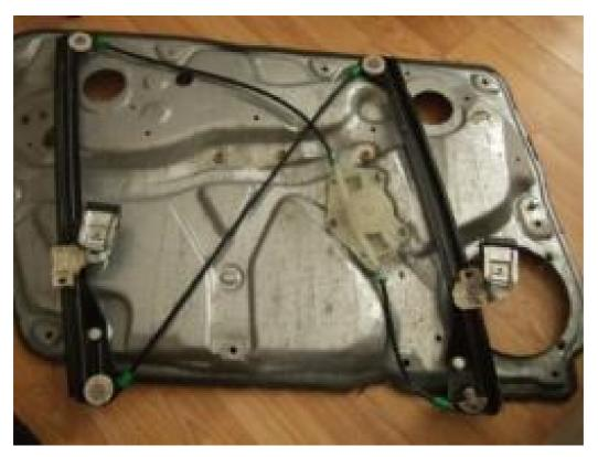
This is an example of the completed repair; note the orientation of the wires and the layout of the plastic cage that holds the reel for the wire
