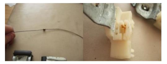
These little notches on the wire need to be placed into the applicable holes on the reels. There is one for both sides of the wire. If the wire has already been fitted, they can still be put on afterwards. It is just a bit tight.
