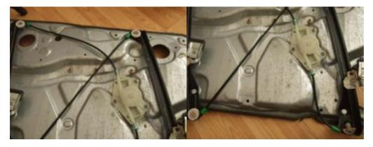
This is a close up example picture of the cable / pulley system for one half of the door panel
