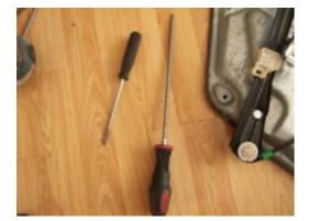
The tools you will need to complete the repair will be a T20 Torx screwdriver and a Flat Screwdriver additionally, you could also use a pair of pliers to remove the plastic plug holding the wire nearest the speaker instead of the screwdriver method.
