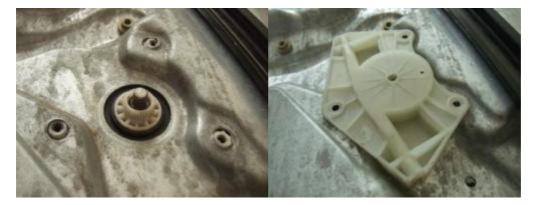
Place the motor on the door panel so the holes line up to the holes for the screws in the panel. Don't worry about fitment, it will physically only fit one way on the panel itself. Once the cables are wired up, you then flip the casing over face down and push the reel onto the teeth of the motor. Once they are pushed on, use the screwdriver and attached it to the face of the motor. It may be loose at first, but will self align when you start screwing it on
