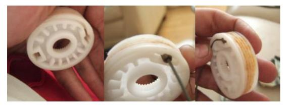
This is the reverse end of the plastic pulley; you thread in the "short" end of the cable into this side and wind it into it (the short end is the one closest to the speaker cable). When you thread the cables you first have to put them in at a 90 degree angle to their storage hole otherwise they won't fit. Once they're in the hole, just rotate them and wind them into the reel as normal make sure it's as tight as possible to avoid slipping on fitment (they will be tight when under tension).
