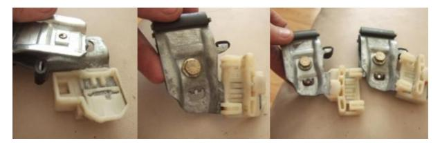
You will receive some new plastic clips which hold the window rests in place, you will need to dismantle the clips from the old one to separate them, these are usually tight so may require breaking to remove them. The new ones push fit into the old rests. Double check everything when fitting and match it up to the window before fitting as they're quite hard to remove and only fit one way.
