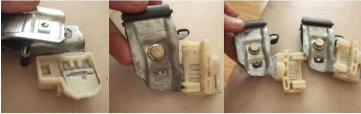
You will receive some new plastic clips which hold the window rests in place, you will need to dismantle the clips from the old one to separate them, these are usually tight so may require breaking to remove them. The new ones push fit into the old rests. Double check everything when fitting and match it up to the window before fitting as they're quite hard to remove and only fit one way.
