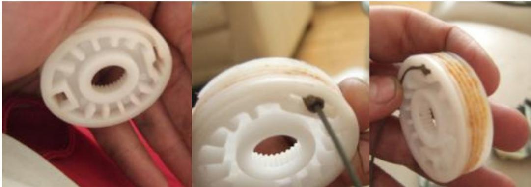
This is the reverse end of the plastic pulley; you thread in the “short” end of the cable into this side and wind it into it (the short end is the one closest to the speaker cable). When you thread the cables you first have to put them in at a 90 degree angle to their storage hole otherwise they won't fit. Once they're in the hole, just rotate them and wind them into the reel as normal make sure it's as tight as possible to avoid slipping on fitment (they will be tight when under tension).
