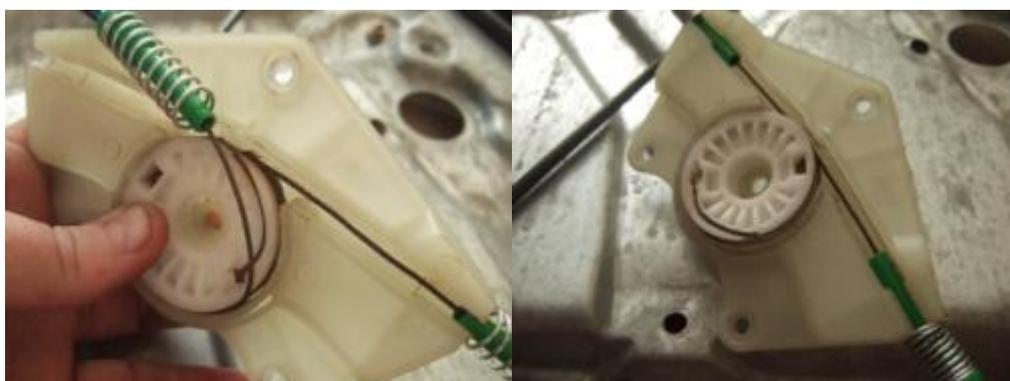
After you have wrapped the wire around the wheel, you will need to put it inside the housing with the inside edge with the teeth facing outwards. You will then need to compress the springs on the plastic tabs against the housing so that everything fits. This step will be **HARD** to some degree if not using a pretensioned kit
