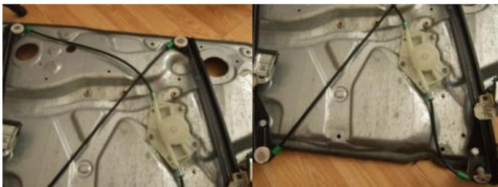
This is a close up example picture of the cable / pulley system for one half of the door panel
