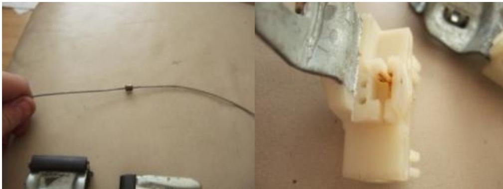
These little notches on the wire need to be placed into the applicable holes on the reels. There is one for both sides of the wire. If the wire has already been fitted, they can still be put on afterwards. It is just a bit tight.
