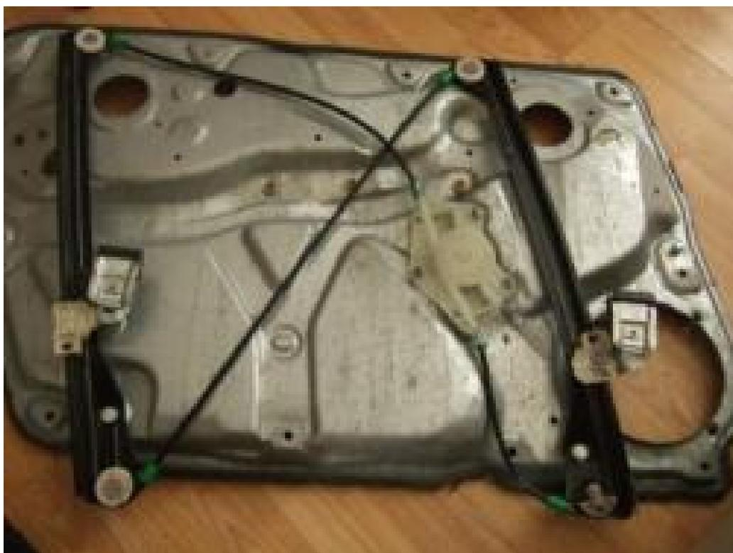
This is an example of the completed repair; note the orientation of the wires and the layout of the plastic cage that holds the reel for the wire
