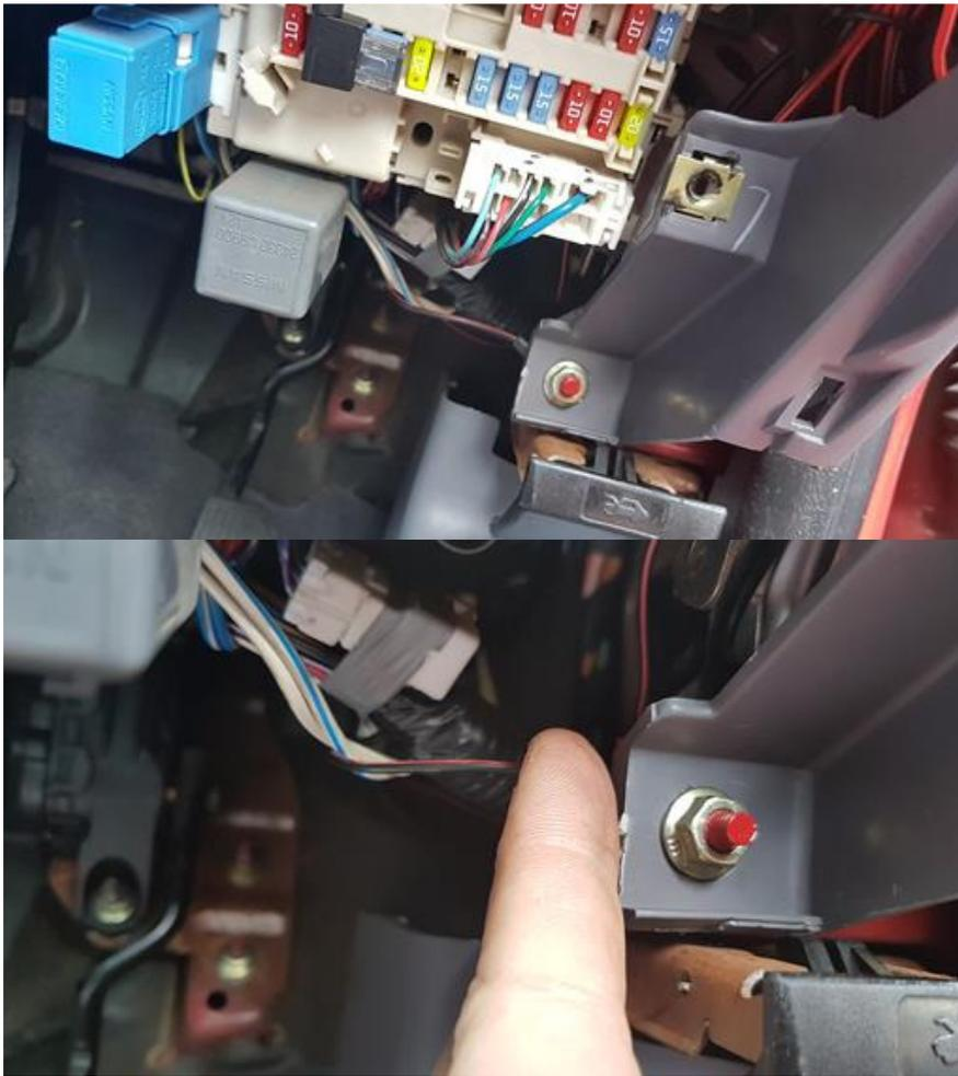
If you had disconnected the battery, reconnect the battery on the car, and put the keys in the ignition then switch it to ACC. Your dashcam should now power up. If all has been done correctly, you just need to reinstall trim (lower shroud, A-pillar and lower storage compartment)
