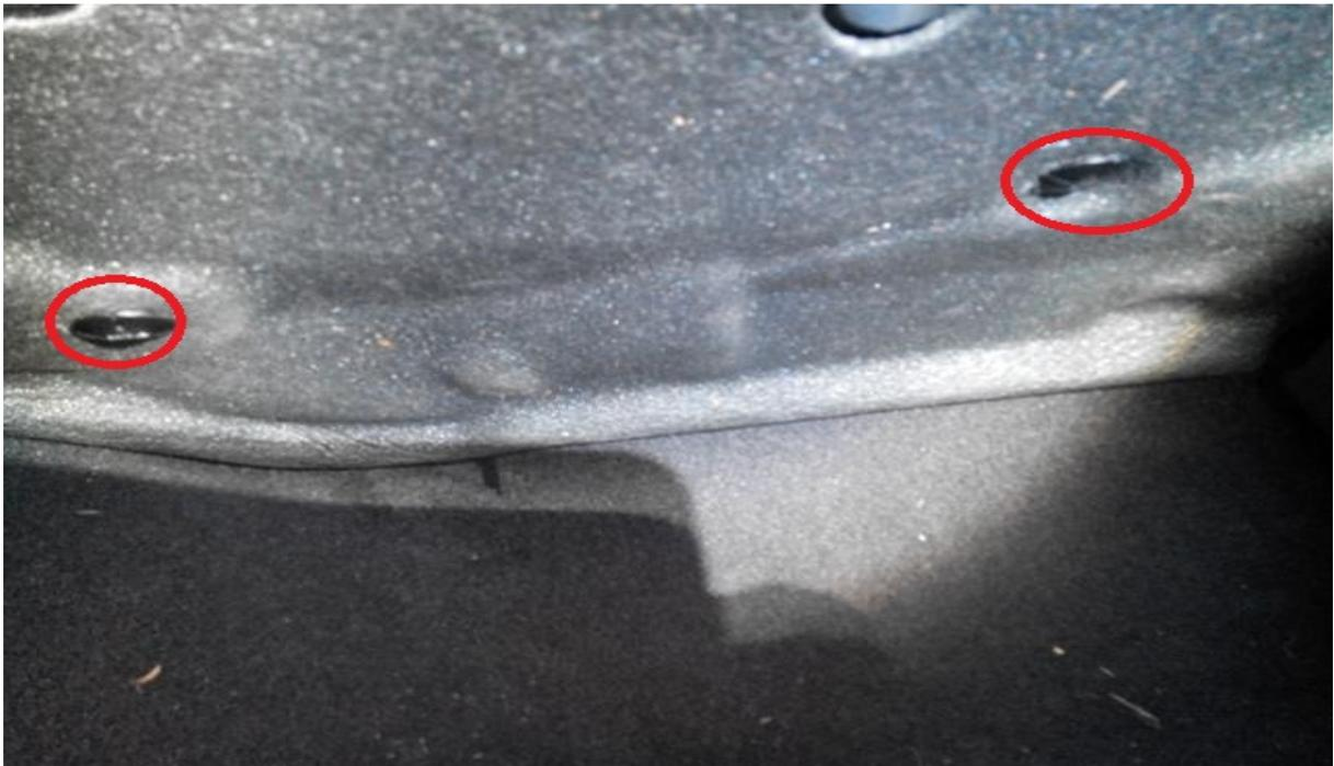
When you have removed the Torx screws, change your bit or changeover to the flat head screwdriver. You will need to look underneath the glove box; you will then see the following two plastic screws holding the foam in place. Remove these screws
