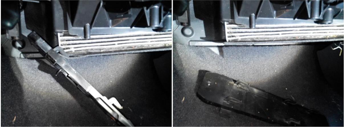
When you have slid the cover off, it will fall down to the floor and the older filter should pull out quite easy enough. You will then be able to see the quality of the filter you are removing on your car after the latch has been released
