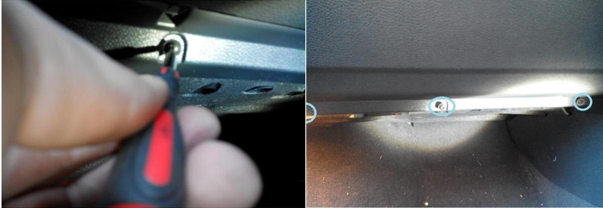
Using your screwdriver with the T20 torx bit, loosen the 3 screws underneath the glove box holding the filter housing and foam cover in place. You can see them circled above in the 2<sup>nd</sup> picture; they're spaced evenly apart, one nearest the centre column, one in the centre and one nearest the door next to the foot well light. Remove these screws
