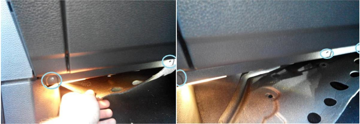
When you have removed the torx screws (I have circled their relevant positions above) and the flathead screws from the foam, you will need to remove the foam away from the covers. I found the best way to do this is by digging a finger just behind the light, there is a gap here. Once you have started moving the foam away it should come off easy if you have removed all 5 screws.
