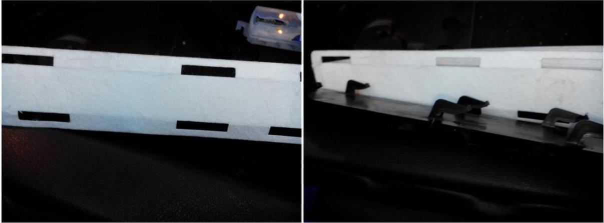
This picture is mainly for reference, this is the latches that the cover for the pollen filters housing slots into when the filter has been reinstalled. The latch will only fit one way, so it should be easy enough to work out. As reinstallation is just simply a case of swapping old for new filters and securing the latch again
