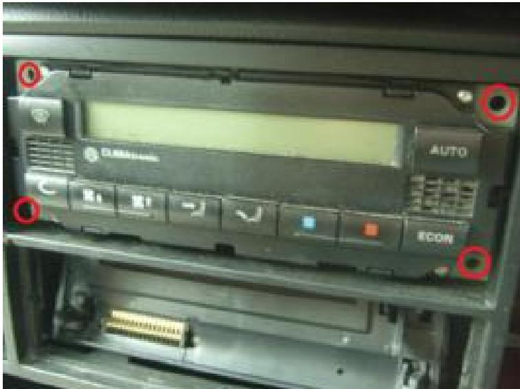
Remove the fascia surrounding the climatronic and disconnect it by popping it off. You will then need to remove the 4 torx screws (T20) – highlighted so that you can remove the climatronic from the dash. Also pop off the hazard switches using the teaspoon method and unclipping the connectors at the back so the wires don't snag on the dashboard when you're removing it.
