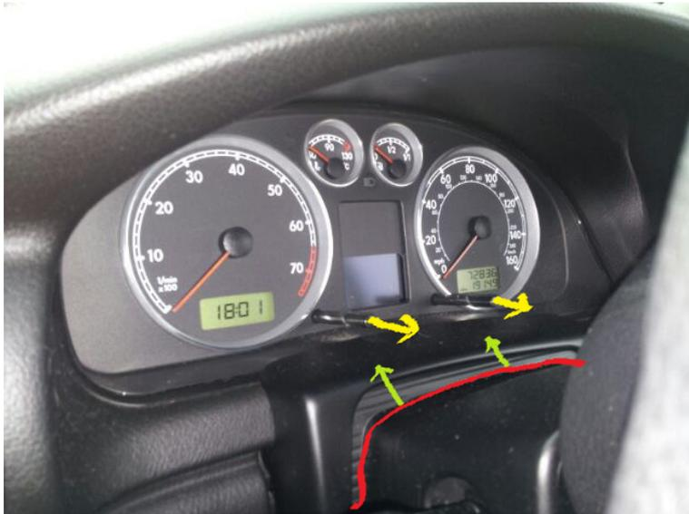
Lift the plastic shutter doors (the red line) in the picture around the steering wheel shroud column. Under this there will be some torx screws that hold the plastic for the shroud and the dash in place against the steering wheel (the green arrows). You will need to remove these. Once the screws are removed and your ready to remove the dash. Hold the screws on the odometer (yellow arrows) and pull forward gently while wiggling it forward until you access the back of the clocks.
