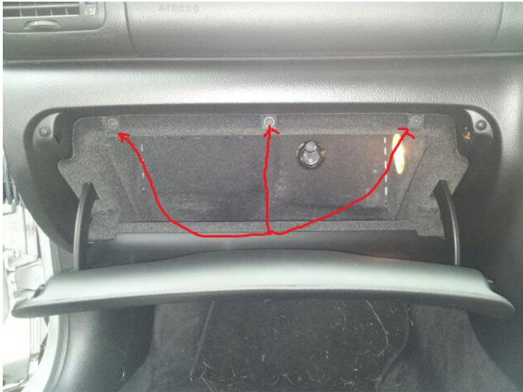
Loosen the 3 torx screws inside the glovebox , this will allow you to remove the glovebox once you have removed the bottom screws from the glovebox.
