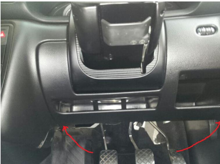
Remove the two lower torx screws underneath the steering wheel column shroud. You will need to crouch down and look up as they're at the back and quite hidden. Although they're easy enough to remove without any issues. Once these are removed you can then remove the lower steering wheel shroud.
